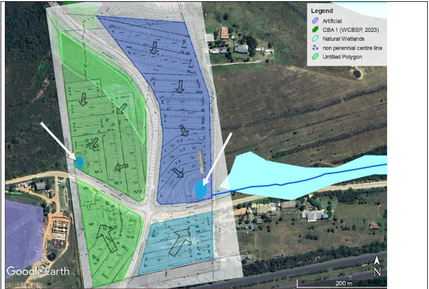
Figure 10: SWMP overlaid showing direction of runoff and indication of proposed SWM ponds (east and western); one artificial wetland will be retained as a SWMP; the artificial wetland in the north central section falling within mapped CBA is recommended to be retained and development not take place within this mapped CBA.
