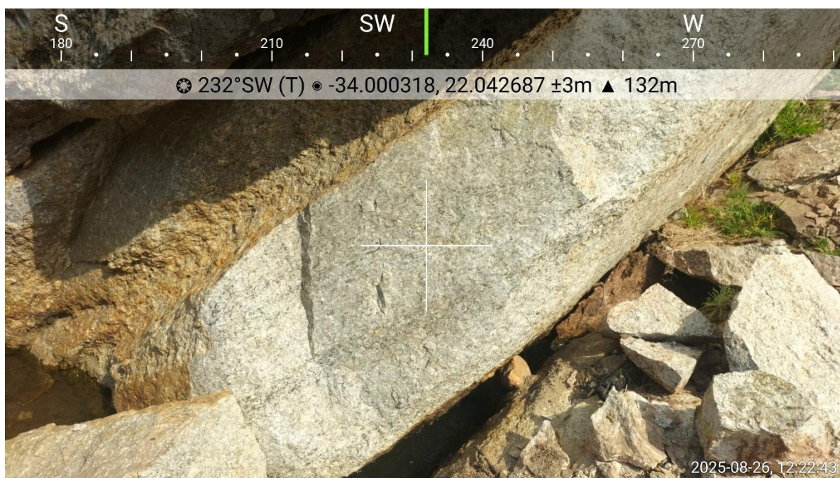
Figure 4-2: Gneissic banding (darker band below the centre cross)
