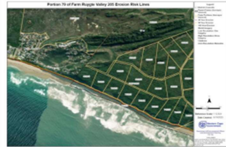
Fig. 4: Erosion risk lines (20, 50 & 100 year) as situated on the southern boundary of Ruygte Valley 205 Portion 79 (DEADP Coastal Management Map viewer).
