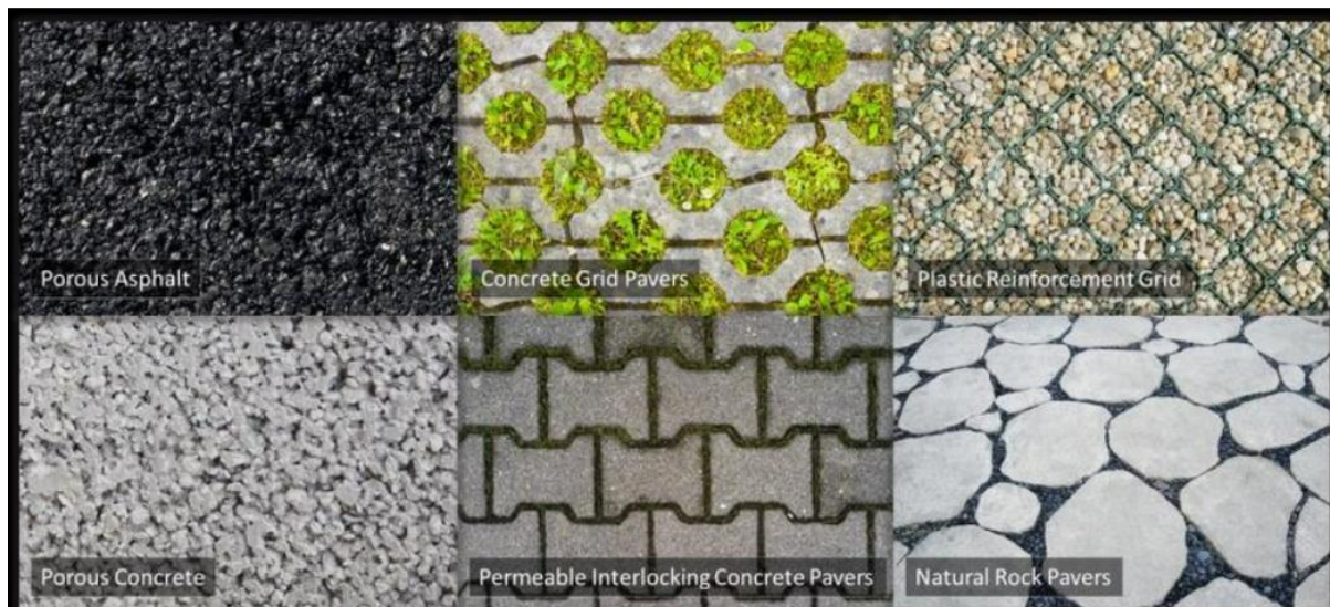
Figure 24. Examples of permeable surface which should be used as an alternative to impermeable paving or road surfaces wherever possible.
