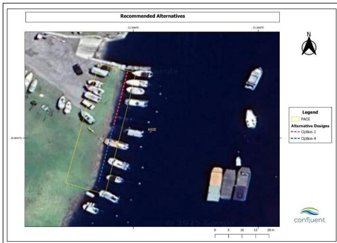
Figure 2: Map illustrating the recommended alternatives options (2 and 4) to be implemented to address bank erosion along the estuary shoreline
