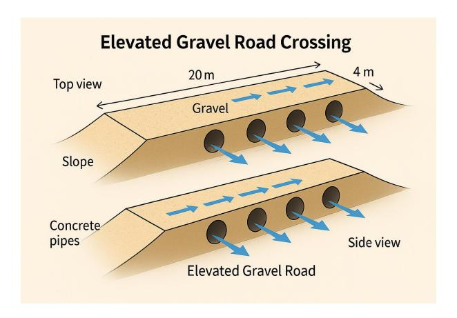
It will also be constructed to avoid erosion in event of heavy rains as shown in the diagram below.
