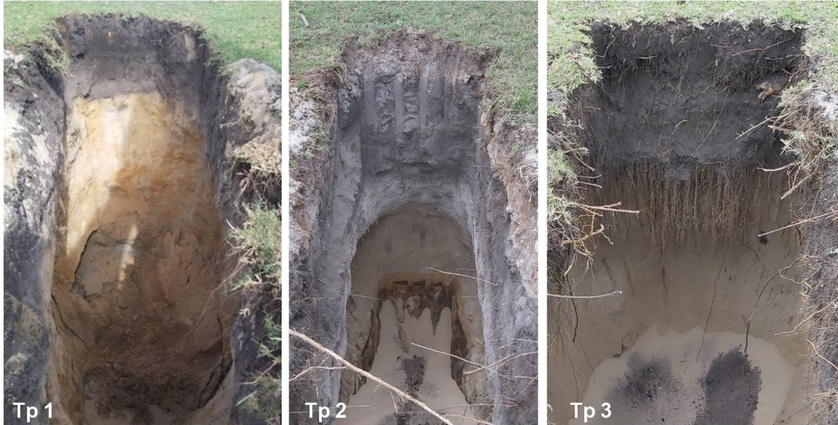
Figure 29. Profiles of geotechnical test pits 1, 2 and 3 on 91/304. The depths from surface to base of excavation are as follows; tp1 = 2 m, tp2 = 2, 5 m and tp3 = 2, 5 m. Courtesy of the client and Outeniqua Geotechnical Services.
