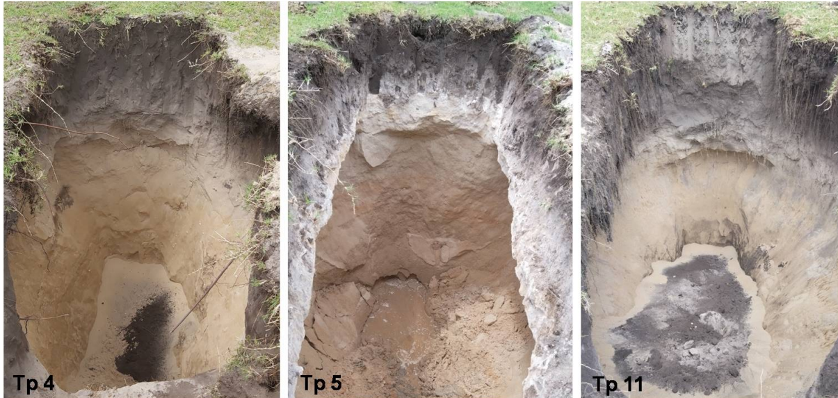
Figure 30. Profiles of geotechnical test pits 4, 5 and 11 on 91/304. The depths from surface to base of excavation are as follows; tp1 = 2, 5 m, tp2 = 2, 5 m and tp3 = 3 m. Courtesy of the client and Outeniqua Geotechnical Services.
