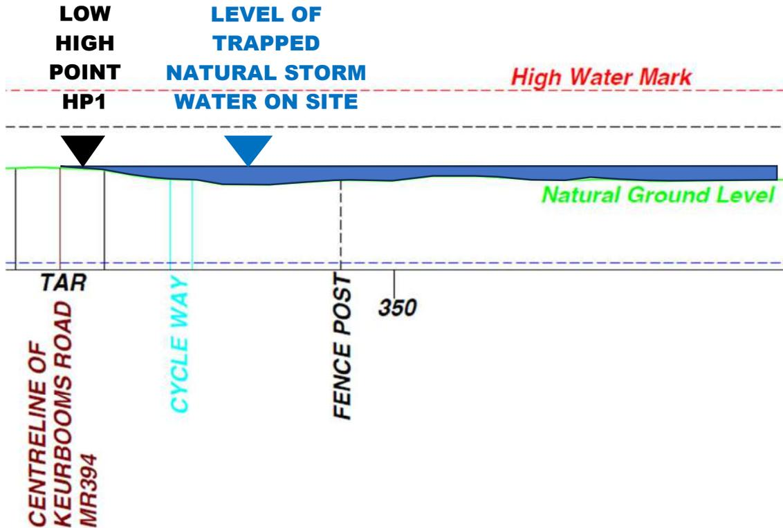
Figure 3F: STORMWATER: PART 1 OF SECTION A-A ENLARGED
