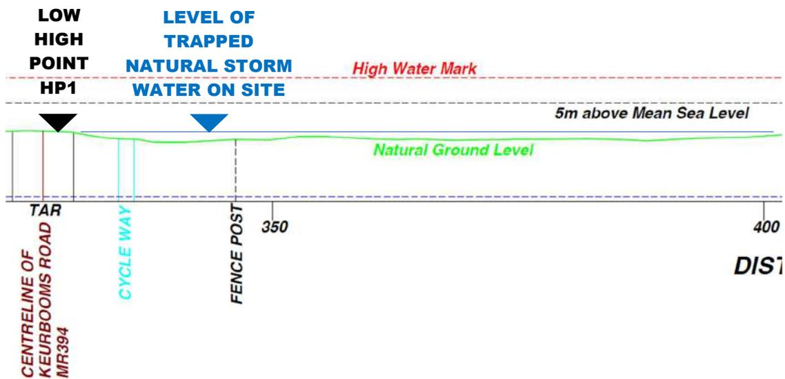
Figure 3C: STORMWATER: PART 1 OF SECTION A-A
