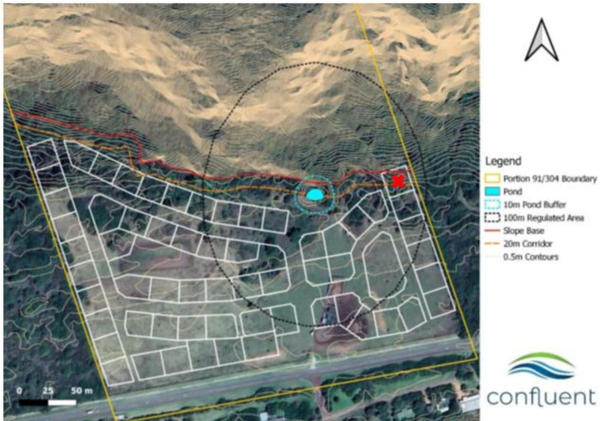
Figure 9: Preferred site development plan overlaid with 0.5 m contours, indicating the pond and buffer, the 100m regulated area of the spring, and the 20m wildlife corridor at the base of the slope. Note that the red X indicates Unit 50 which was subsequently moved back and out of the wildlife buffer (Aquatic Report Figure 18, Appendix 1)
