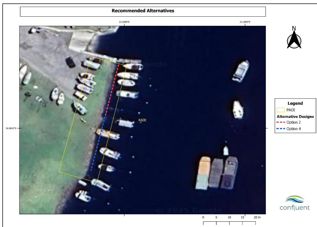
Figure 15: Map illustrating the recommended alternatives options to be implemented to address bank erosion along the estuary shoreline.
