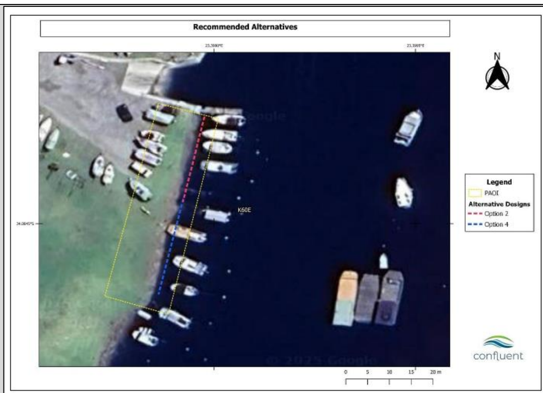
Figure 2: Map illustrating the recommended alternatives options (2 and 4) to be implemented to address bank erosion along the estuary shoreline
