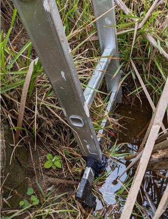
Water measured at between 1.5m and 1.8m below ground level on property opposite site of proposed development.
