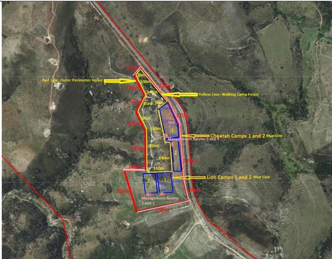
Figure 5: Layout of the Camps: Outer Perimeter, Walking Camp and Holding Camps. Marked in pink are current fence lines. Numbered in pink are where the Management Rooms will be constructed.
