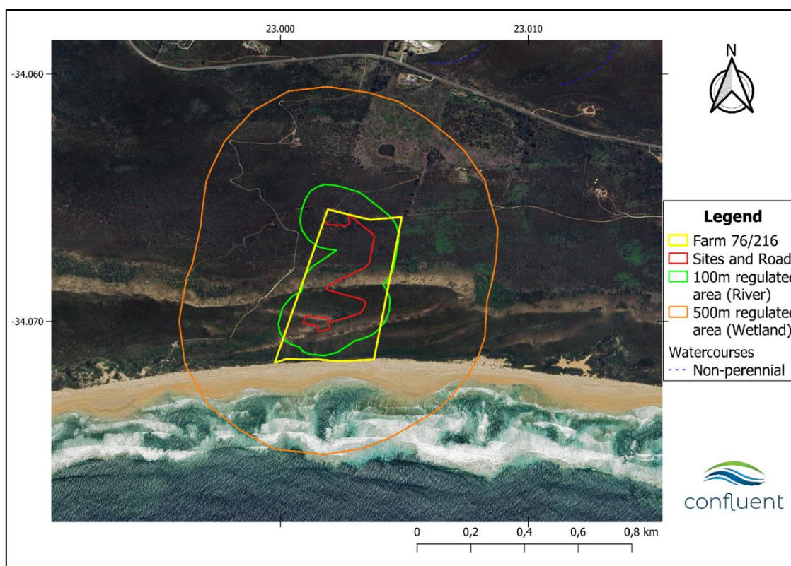
Figure 11: Map indicating no mapped watercourses within 100 m or 500 m from the proposed development site.
