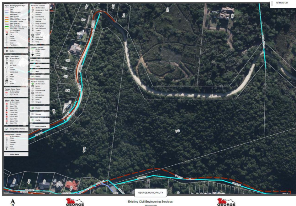
Figure 9: Existing Municipal services. 50mm diameter water connection (blue) and 160mm diameter sewer line (red dashed).
