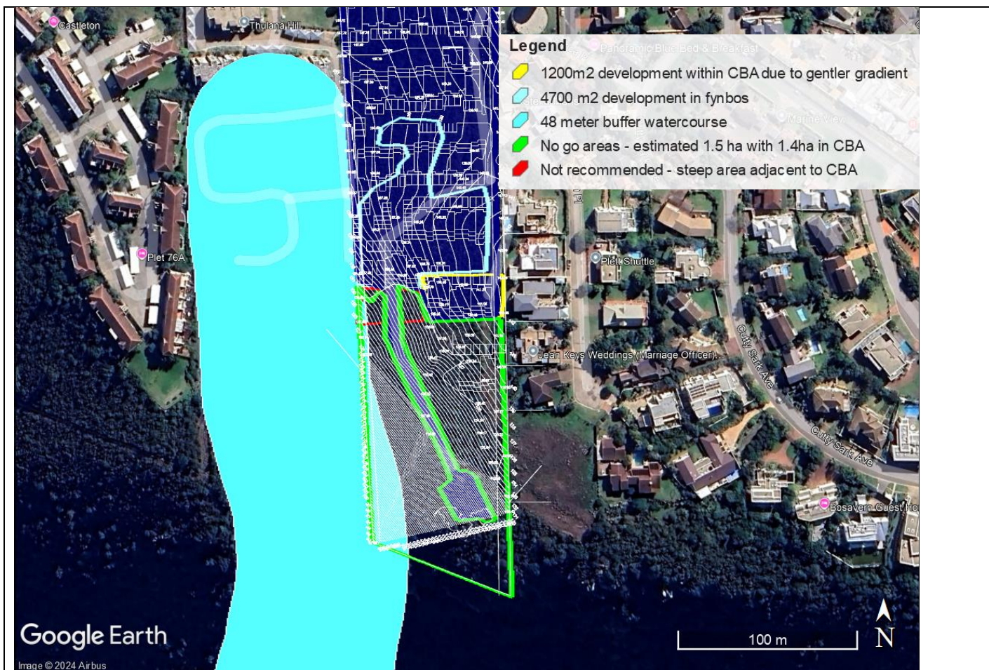
Figure 15: Southern section of development showing 48 meter buffer which coincides with recommended steeper no-go area
