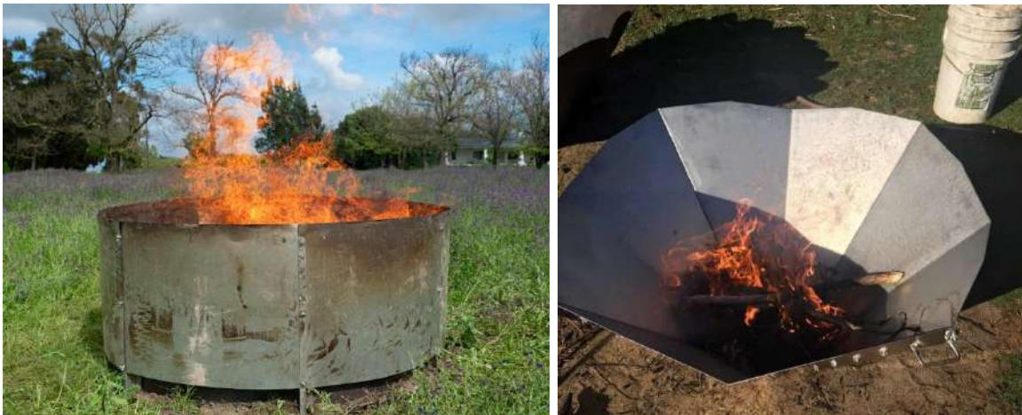
Figure 22: Two examples of biochar kilns that can be used. These kilns can be set up in a disturbed area away from flammable fynbos on Erf 2074.
