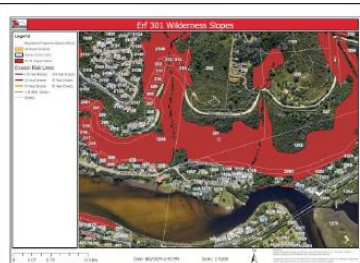
Fig. 10: Slopes on property showing 25-90 degree slopes in sections. George Municipality GIS viewer, August 2024.
