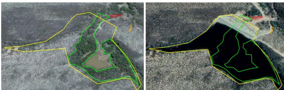
Figure 9. Enlarged dam shown pre- and post-construction with impacted aquatic habitat overlaid. Green = riparian vegetation, yellow = enlarged dam footprint, Orange = sand discard in wetland, and Red = rock discard in drainage line.
