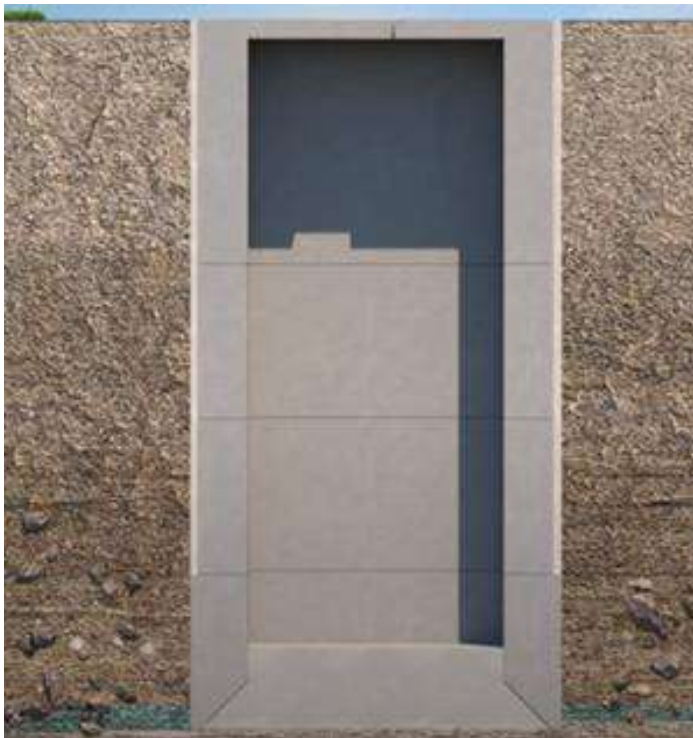
Figure 4-6: A Complete Caisson method
