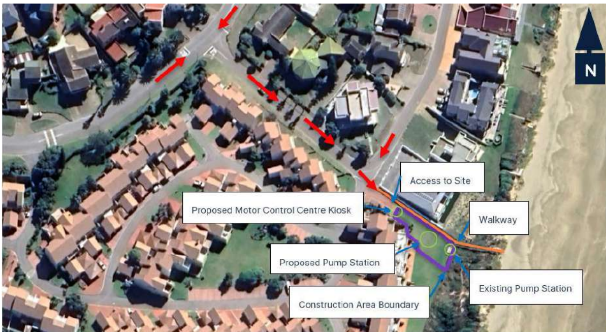
Figure 10: General layout of construction activities
