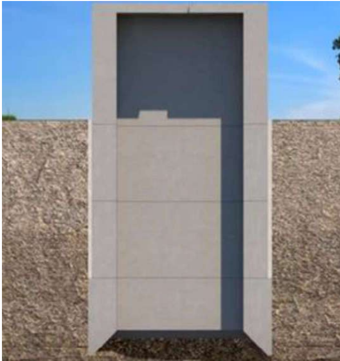
Figure 4-5: Placing of more Concrete rings
