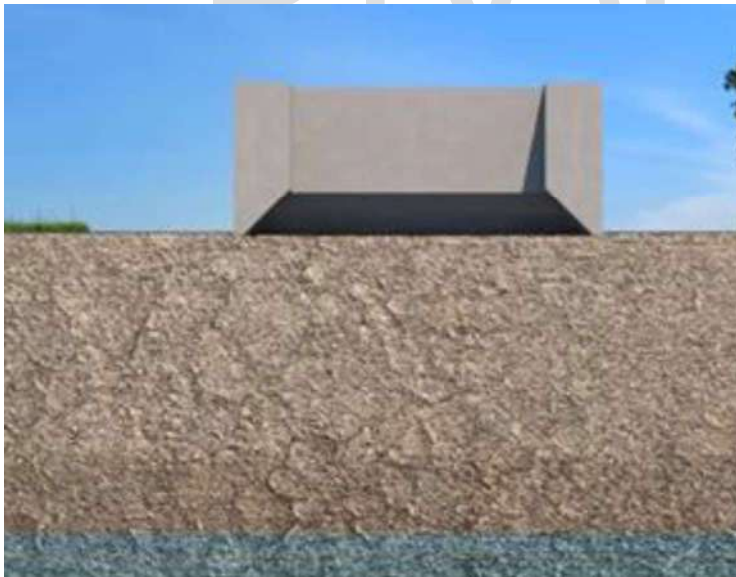
Figure 4-2: First Concrete Ring Placement
