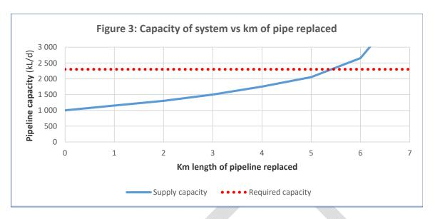
Roughly 5,5 km of the existing 7,7 km x 150 mm Ø bulk pipeline between the Town reservoirs and the Keurbooms River should be upgraded in order to supply the Matjiesfontein reservoir from the Town reservoirs under gravity (no augmentation of bulk supply from the Goose Valley reservoir will then be required).
