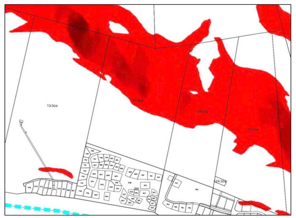
Slope Analysis from KELASP - slopes steeper than 1:4
