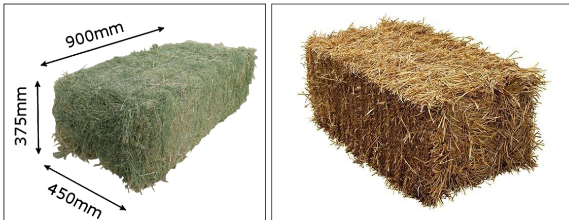
Figure 7. Typically available bale dimensions (left) and a typical straw bale (right).
