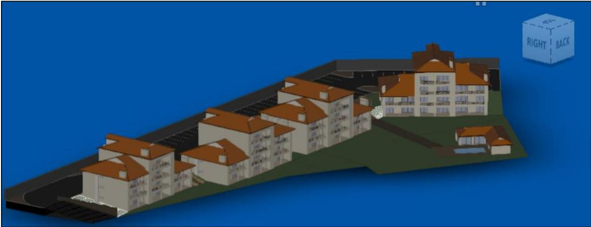
Figure 21. AutoCad 3D model provided by the architect used for rendering the four blocks used as potential architectural design but could change within the 22mamsl tower block/ 19mamsl remaining build height restrictions.
