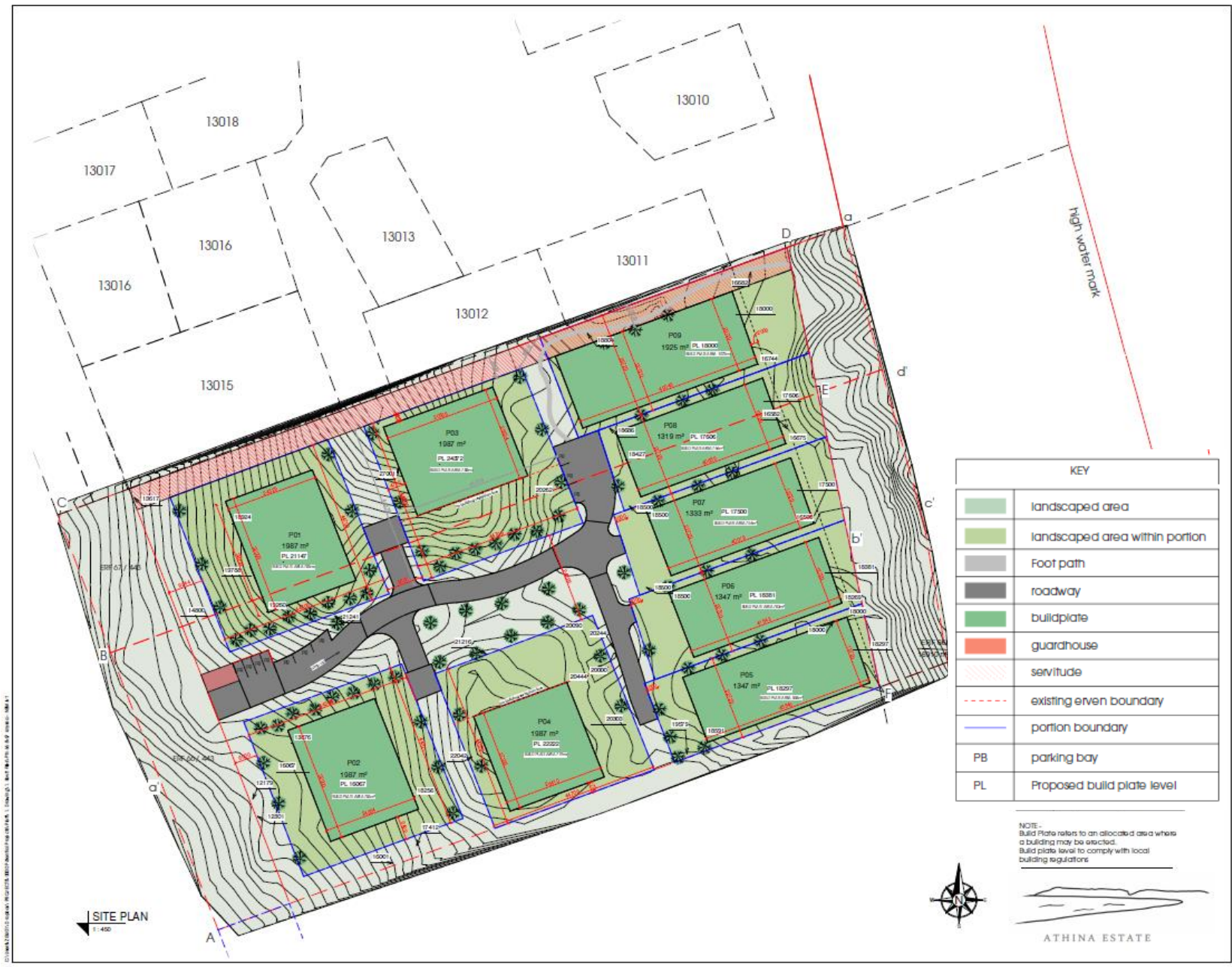
Figure 3: The proposed scheme layout. (The pink hatched area on the northern boundary is a right of way servitude in favour of Portion 60 as described in Condition D of the Title deed of portion 67
