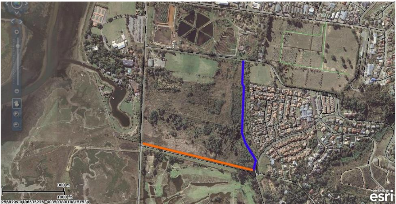
Figure 3: Channel to be excavated using heavy machinery (orange line) and section to be cleared by hand (blue line).
